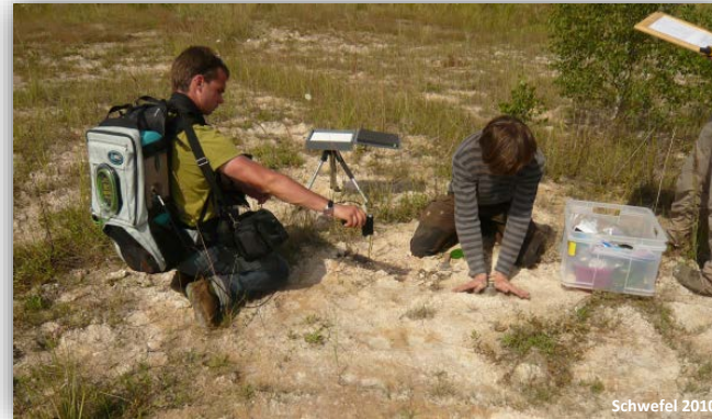
Spectroscopic field measurements and field sampling during summer 2010. The ASD FieldSpec is placed in a backpack.
