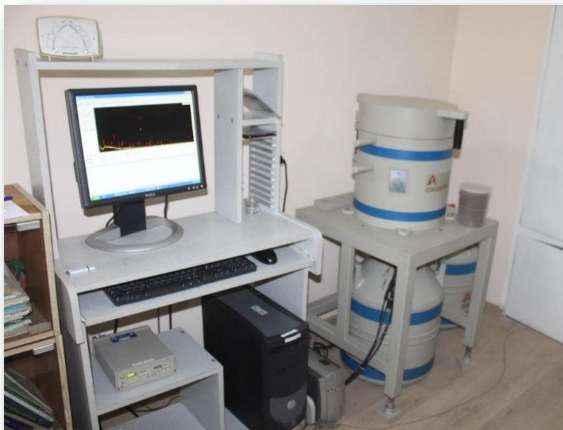
Gamma spectrometry system by CANBERRA
