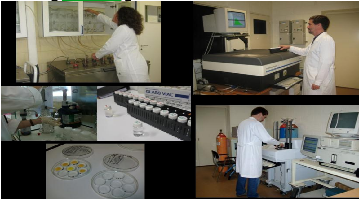
Preparation and measurement of drinking water samples for the determination of radionuclide concentrations and total alpha and beta activity.
